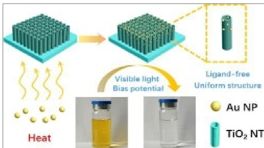
Fig 2: Ligand Free TiO 2 Nano-composites assisted by solar and UV Visible Light potential for purification. (Image Adapted from Reference)
