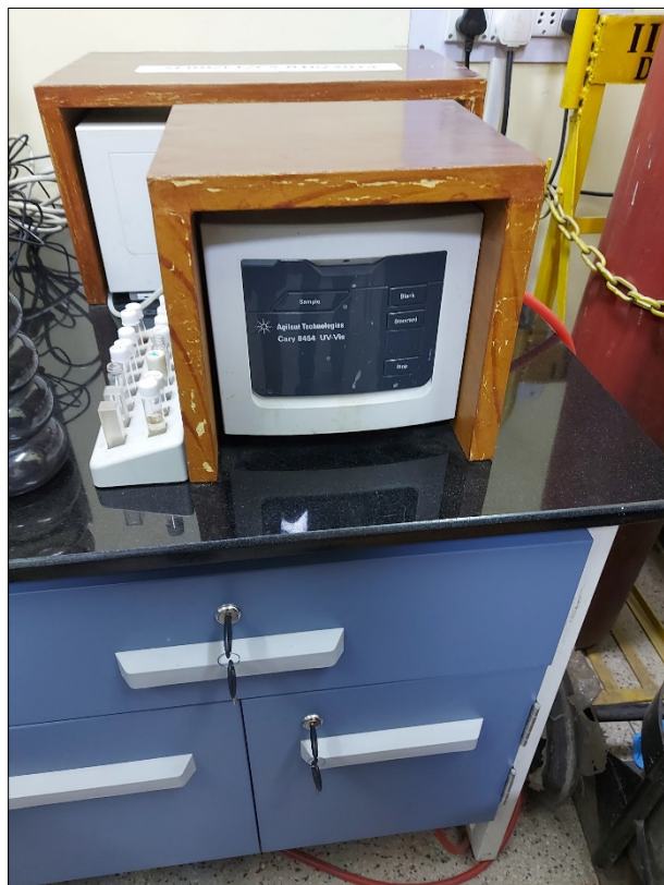
Fig 3: UV Visible Light Spectrometer for potential for purification of Sample. (Adapted from IIT (ISM) DHANBAD Synthesis Laboratory)
