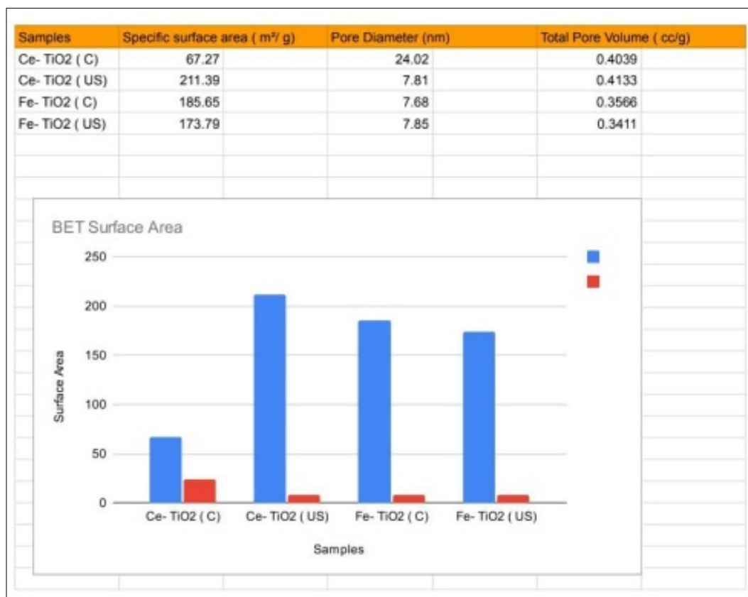
Fig 35: BET Surface Area Curve for Various TiO 2 doped Nanocatalysts
