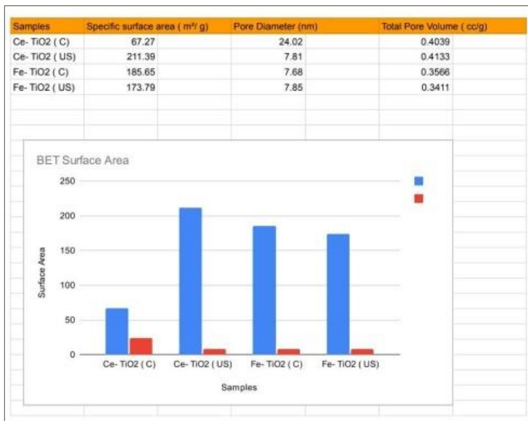
Fig 35: BET Surface Area Curve for Various \text{TiO}_2 doped Nanocatalysts
