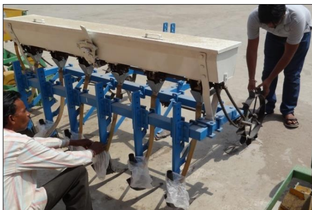
Fig 1: Calibration of fertilizer applicator in the laboratory
