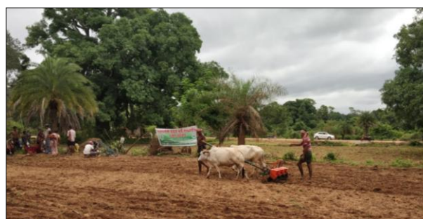
Fig 1: Demonstration of Bullock drawn CIAE 3 row seed drill for line sowing green gram seeds in farmers' field in Mohana, Gajapati
