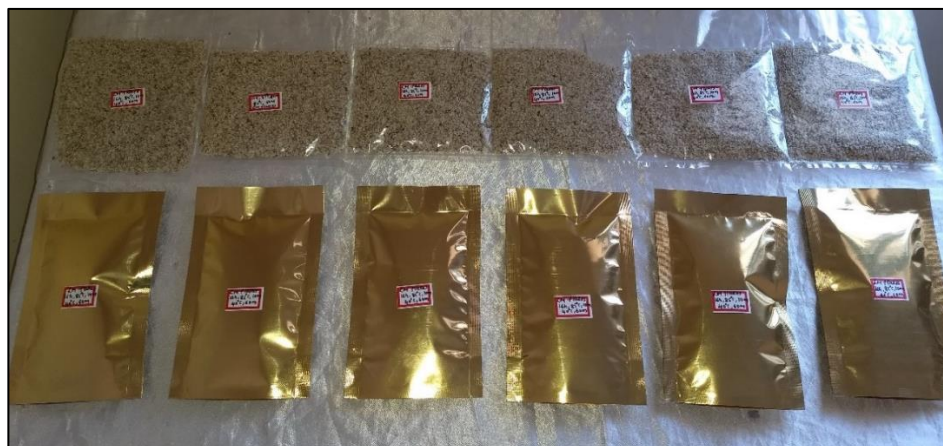
Plate 1: Shelf life study of optimized flakes using metalized polyester and polypropylene
