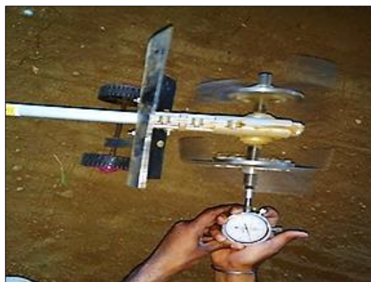
Fig 12: Measurement of rpm of rotor shaft with tachometer
