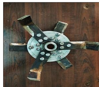
Fig 3: Flange with 6 blades
