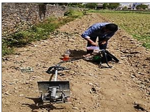
Fig 9: Measurement of fuel consumption
