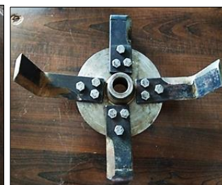
Fig 2: Flange with 4 blades
