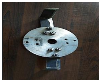
Fig 1: Flange with 2 blades
