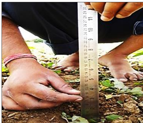
Fig 5: Measurement of depth of cut
