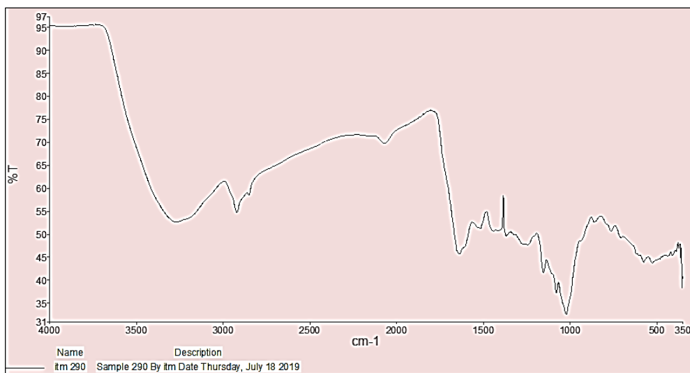
Fig 5: FT-IR spectra of biosynthesised silver sulphide nano particles (1:1 ratio)
