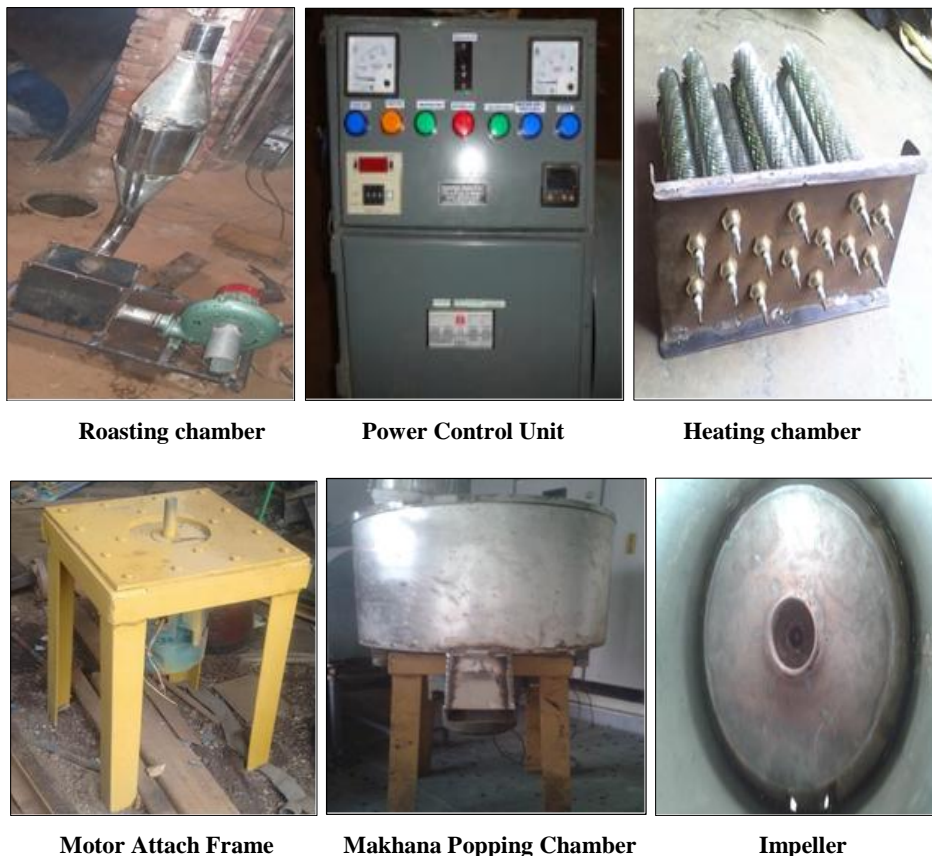
Fig 1: Different components of makhana popping machine
