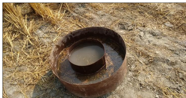
Fig 2: Double ring infiltrometer installed at experimental site
