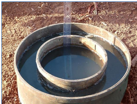
Fig 1: Measurement of field infiltration rate
