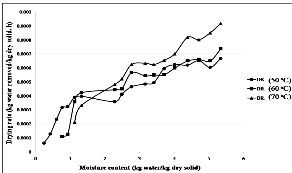
Fig 3: Variation of drying rate with moisture content at different temperatures.
