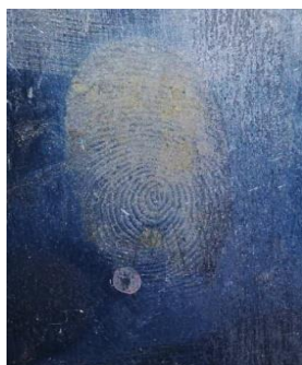
Fig 1: Iodine fuming method showing the latent fingerprint on aluminium surface at 5 °C.
