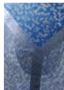
Fig 6: Small Particle Reagent showing the latent fingerprint on plastic surface at -5 °C
