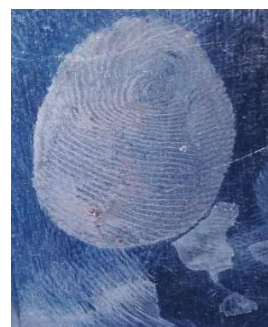
Fig 3: Silver Nitrate method showing the latent fingerprint on aluminium surface at 0 °C
