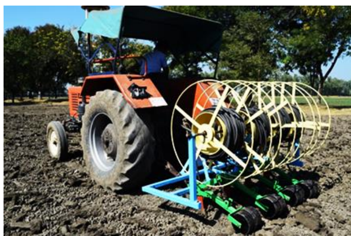
(a) Developed Sub-surface drip lateral laying machine (b) Experimental layout laid by the machine
