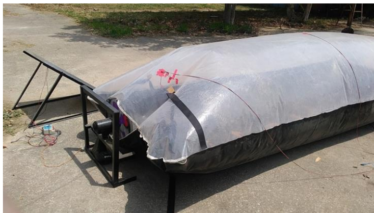
Fig 1: Developed solar powered air inflated grain dryer
