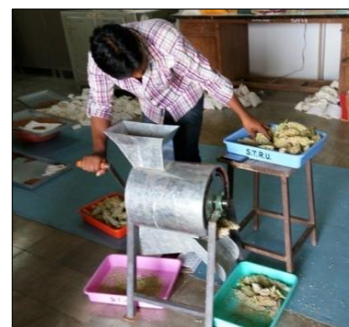
Plate 3: Hurda extraction machine in operation
