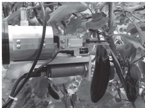
Fig 3: The end-effector of the eggplant-harvesting robot
