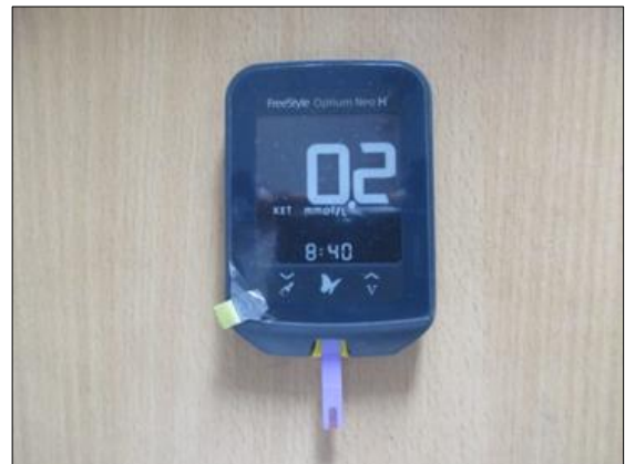
Fig 1: Blood \beta -hydroxybutyric acid (BHBA) concentration determination using a handheld portable human blood ketone and glucose monitoring system (Free Style Optium Neo H – Abbott ® )
