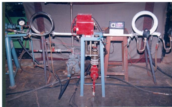
Fig 1: Helical triple tubes UHT milk sterilizer set-up
