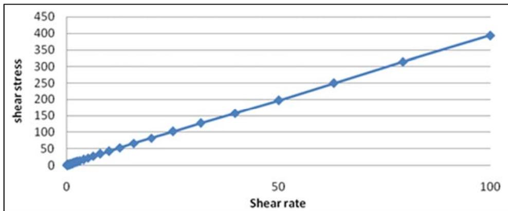
Fig 3: The shear rate V.S shear stress of *Acacia oerfota* gum
