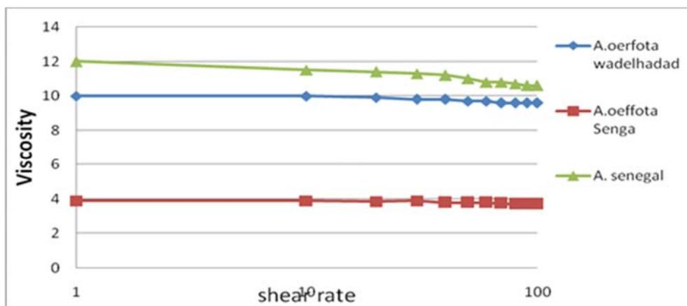
Fig 4: Viscosity profile of *Acacia* gum solution with shear rate - concentration 25%
