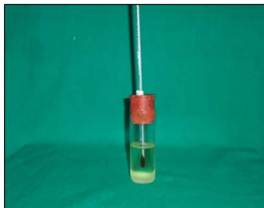
Fig 6: Measurement of cloud and pour point of selected fuel types
