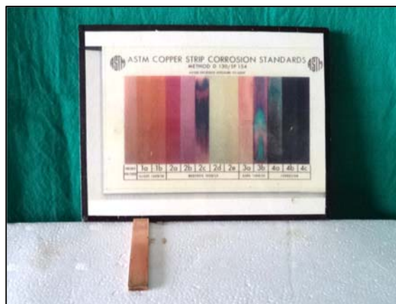
Fig 14: Matching of copper strip colour with the standard chart
