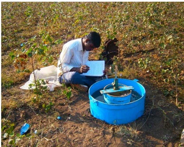
Measurement of infiltration rate in the study area
