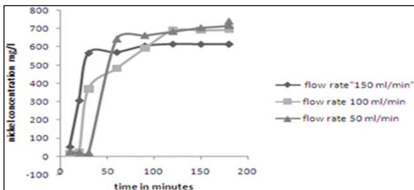
Fig 1: Effect of Flow Rate on nickel Removal
