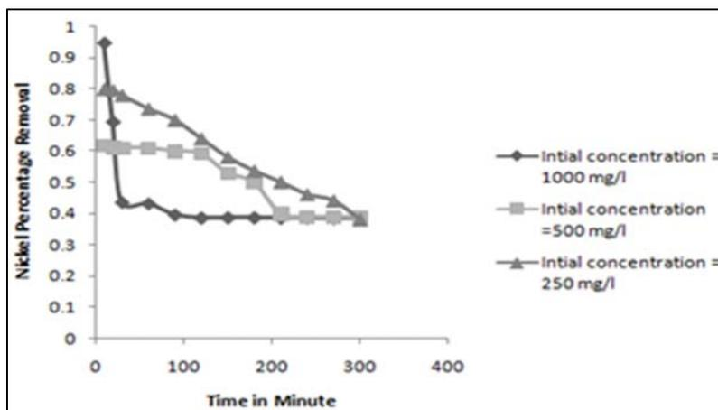
Fig 2: Effect of Initial Concentration on Nickel Removal
