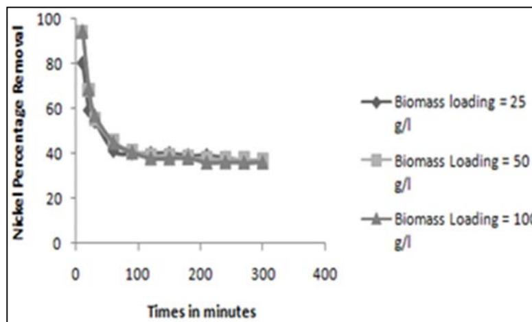
Fig 4: Effect of FPC on Nickel Removal
