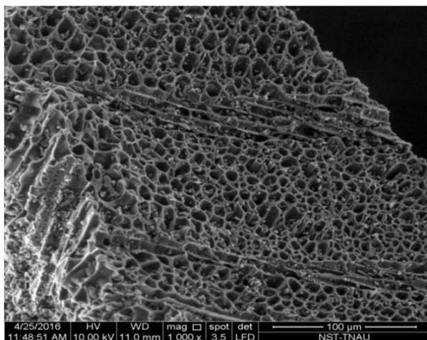
Fig 1: Scanning Electron Microscope of coconut shell biochar
