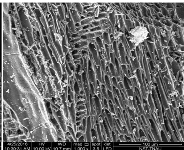
Fig 2: Scanning Electron Microscope of mesquite wood biochar
