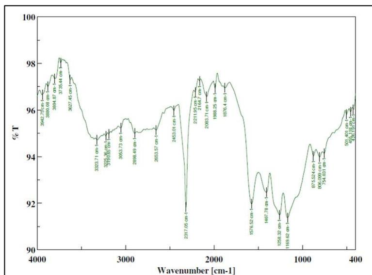
Fig 3: FTIR spectra of coconut shell biochar
