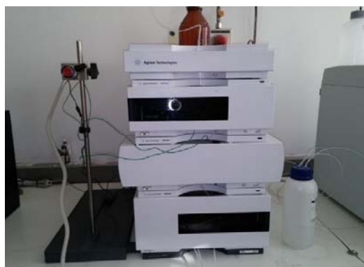
Fig 3: HPLC Device using to evaluation of catalyst
