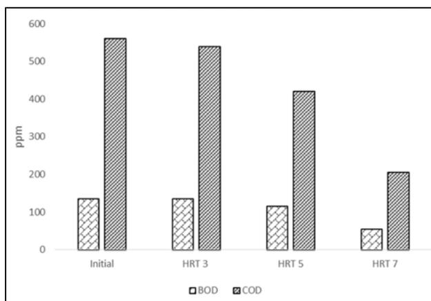
Fig 2: BOD and COD removal efficiency of HRB system
