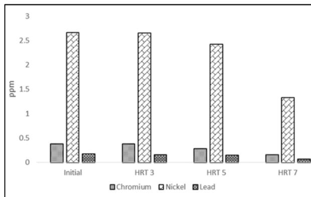
Fig 3: Heavy metal (Chromium, Nickel and Lead) removal of HRB system
