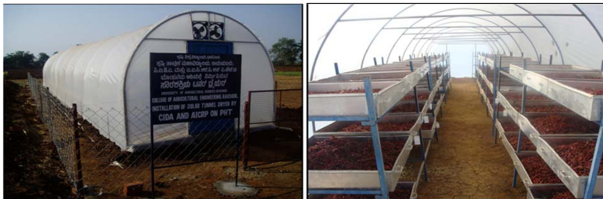
Plate 1: Photographs showing solar tunnel drier designed for chilli drying
