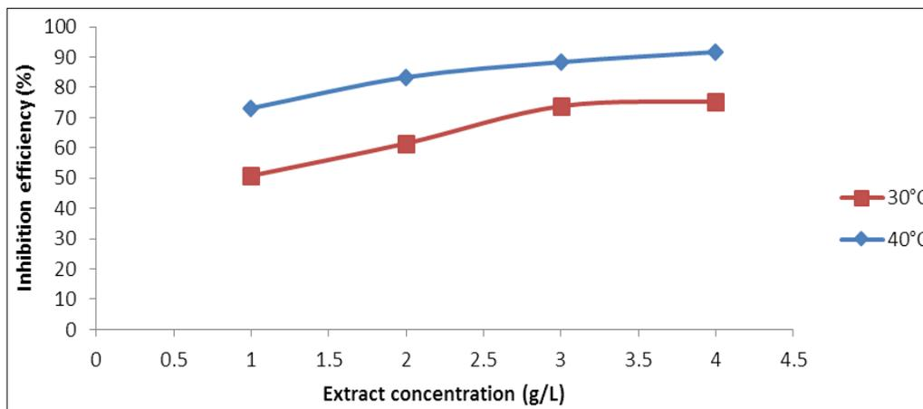
**Fig 1:** Effect of *Commelina diffusa* leaf extract concentration on the inhibition efficiency of aluminium corrosion in 2 M HCl solution at 30°C and 40°C (weight loss measurements)
