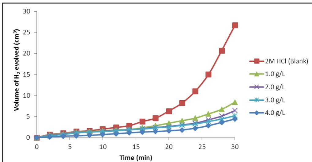
**Fig 2:** Variation of volume of H<sub>2</sub> gas evolved (cm<sup>3</sup>) with time (min) for aluminium corrosion in 2 M HCl in the absence and presence of *Commelina diffusa* leaf extract at 30°C
