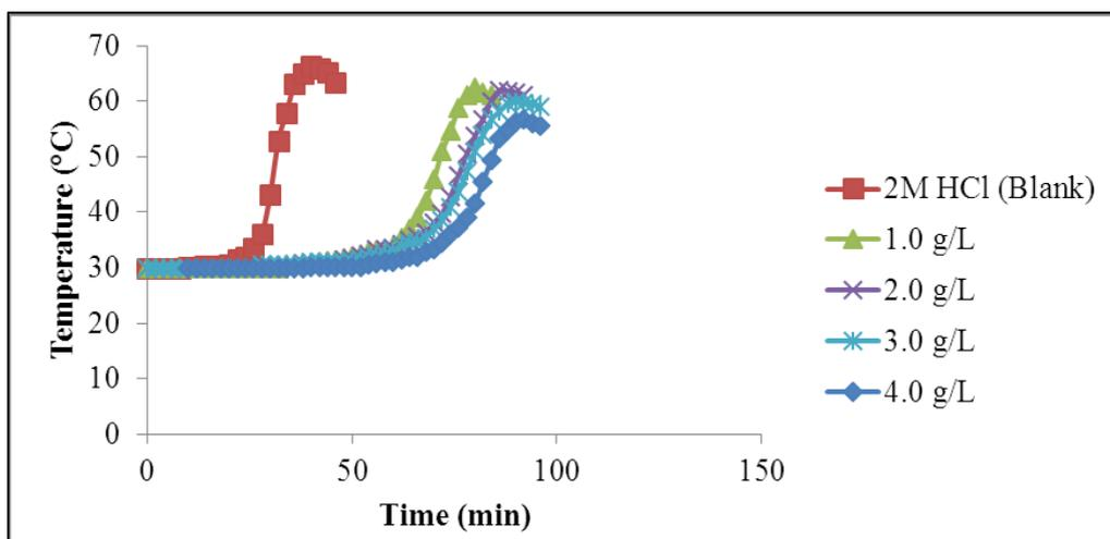
**Fig 3:** Variation of temperature (°C) with time (min) for aluminium corrosion in 2 M HCl in the absence and presence of *Commelina diffusa* leaf extract
