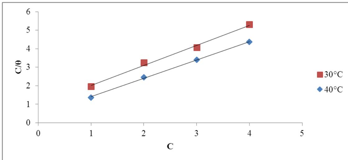
Fig 4: Langmuir isotherm plot for the adsorption of *Commelina diffusa* leaf extract onto aluminium in 2 M HCl solution at 30°C and 40°C
