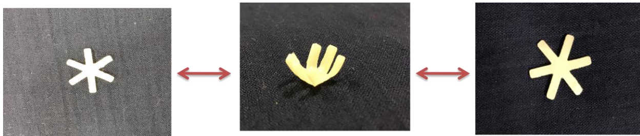
Fig 1: reversible shape memory polymer of poly octylene adipate
