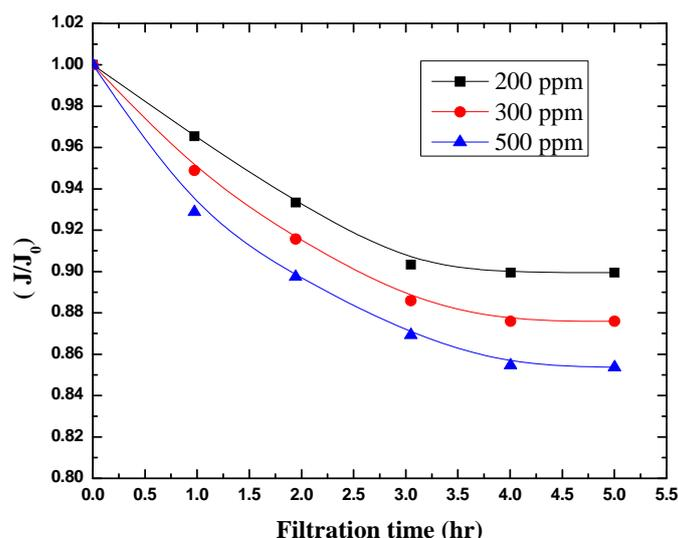
Fig 3.2: Flux Decline with different concentration of sodium alginate.
