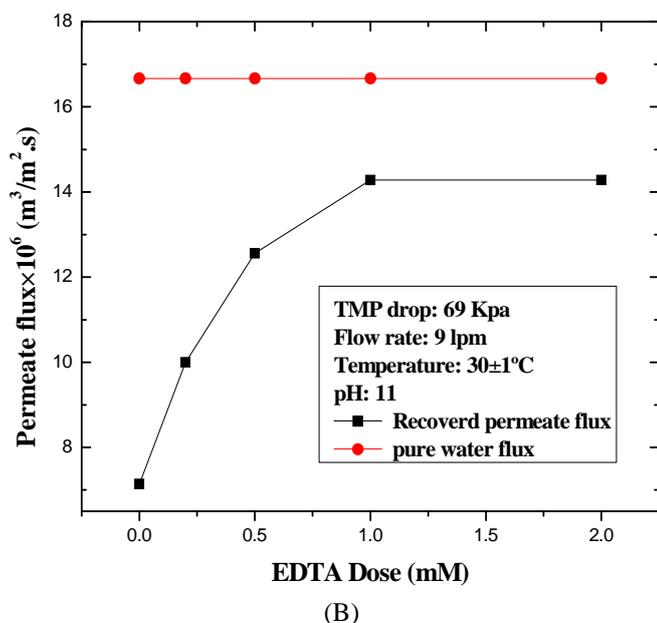
Fig 3.3: Optimization of SDS and EDTA concentration to recover the permeate flux.
