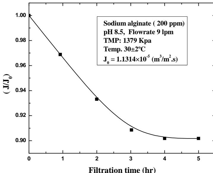
Fig 3.1: Flux behaviour during the organic fouling of RO membrane
