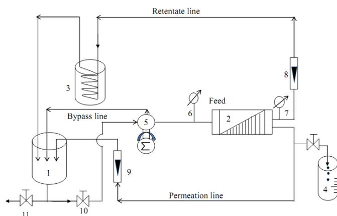
Fig 2.1: Schematic diagram of spiral wound membrane setup
