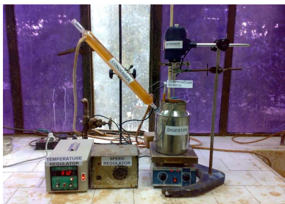
Fig 1: experimental set up for leaching study
