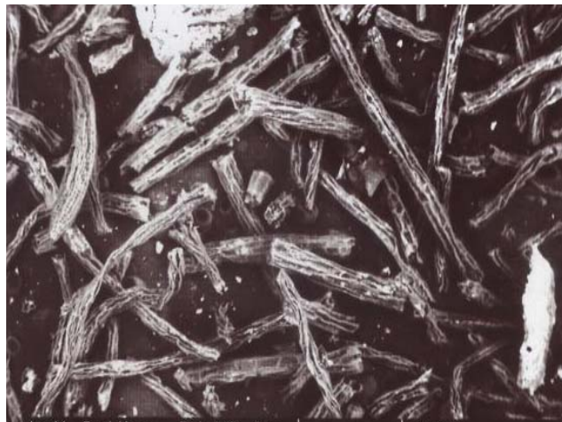
Fig 4C: SEM of TBP-WHR after uranium adsorption.
