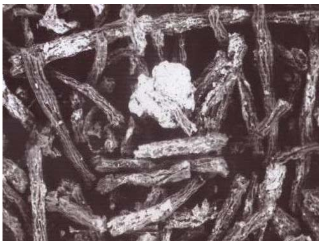
Fig 4A: SEM of WHR after uranium adsorption.
