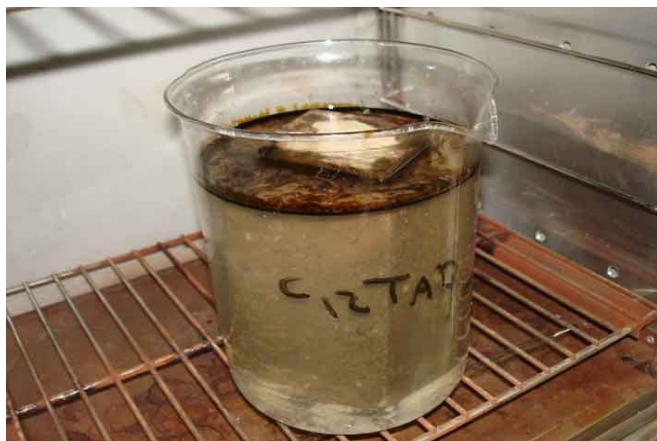
Fig 10: Spontaneous imbibition and oil recovery from reservoir rock in the presence of an optimal solution of C 12 TAB at 70 °C after 48 h
