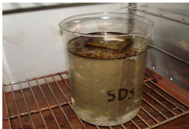
Fig 9: Spontaneous imbibition and oil recovery from reservoir rock in the presence of an optimal solution of SDS at 50 °C after 48 h
