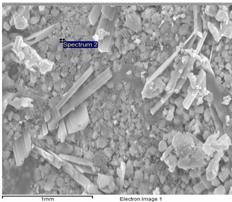
Fig 5: Spherical particle-like phase for EDS study.
