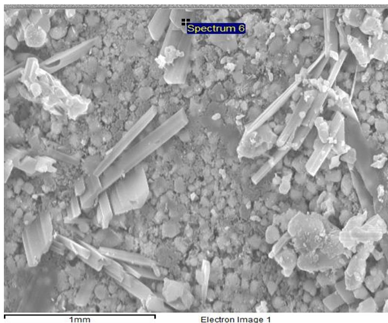
Fig 7: Broken brick block-like phase for EDS study.
