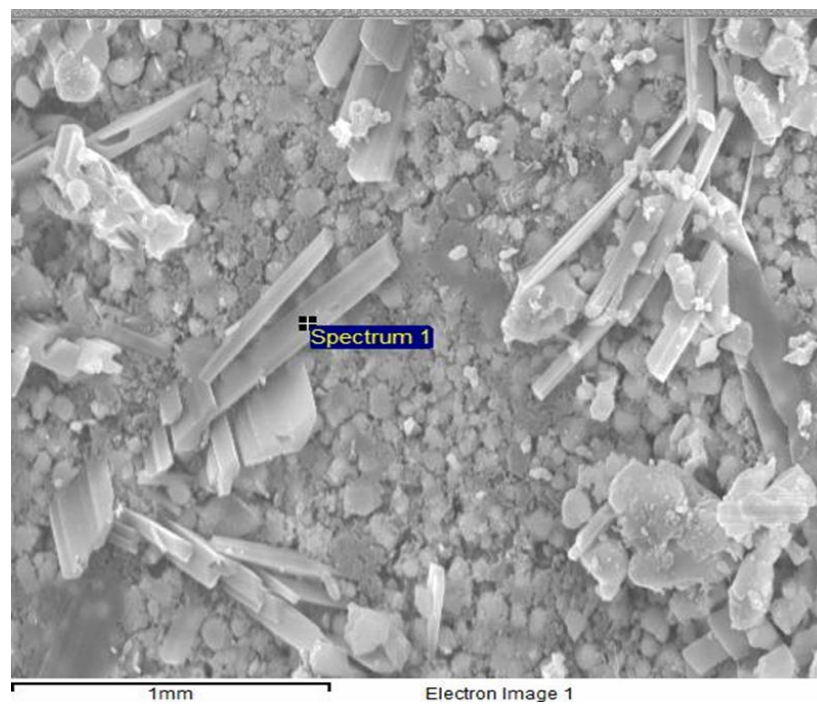
Fig 4: Rod-like phase for EDS study.
