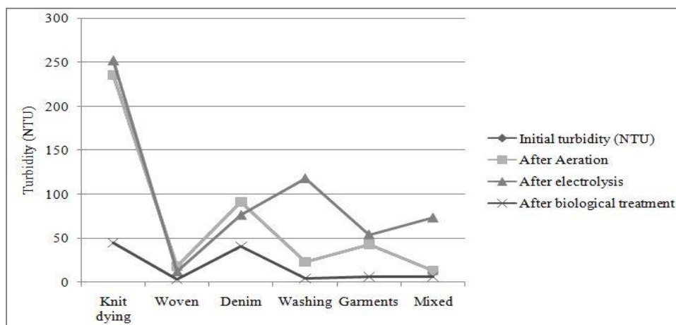
Fig 5: Effect of electro coagulation and biological process to reduce turbidity
