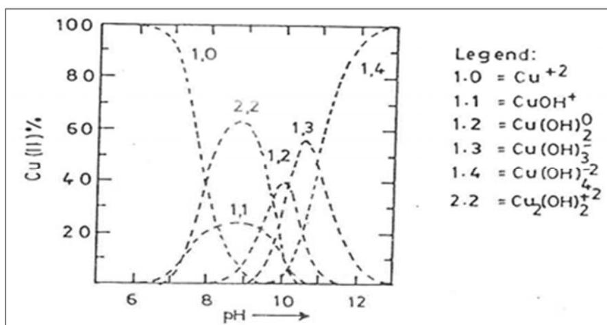
**Fig 16:** Speciation of Cu(II) with varying pH
