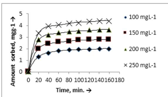
Fig 5: Effect of contact time on adsorption of Cu(II)
