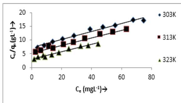
Fig 9: Langmuir isotherm for adsorption of Cu(II)
