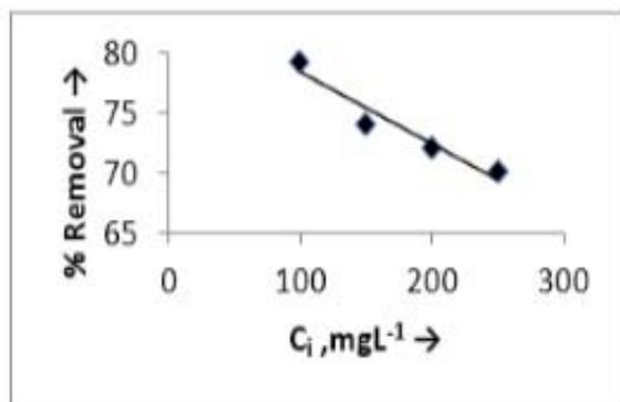
Fig 3: Effect of initial conc. on Cu(II) adsorption
