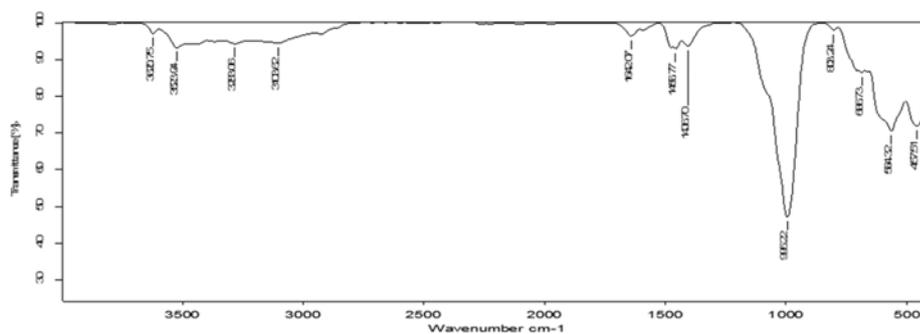
Fig 2(a): FTIR before adsorption
