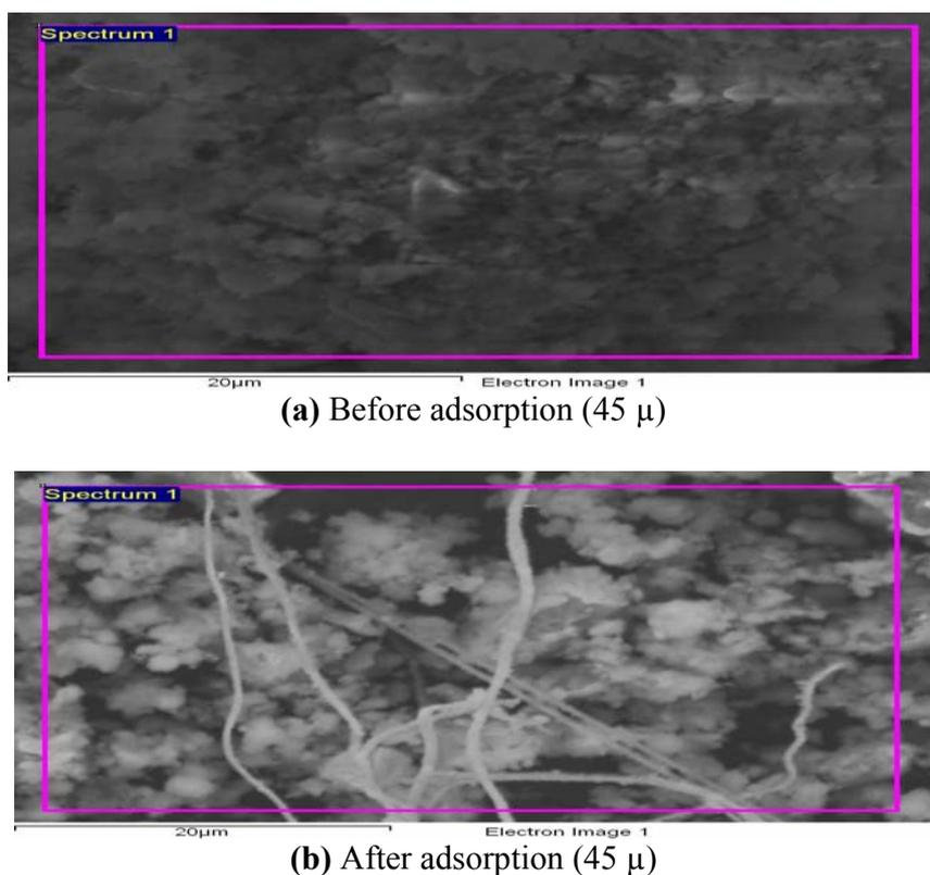
**Fig 1:** (a) is the SEM image of red mud before adsorption and 1(b) after adsorption.
