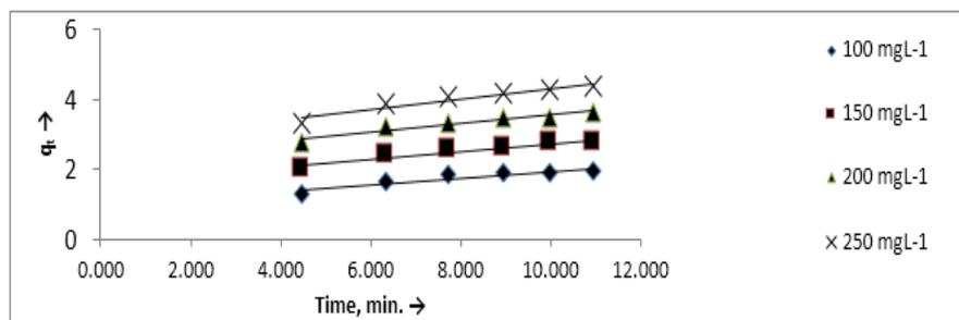
**Fig 13:** Intraparticle diffusion model for adsorption of Cu(II) ion on red mud
