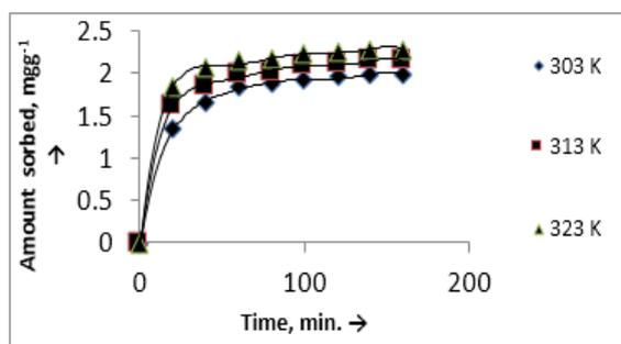
Fig 7: Effect of temperature on adsorption of Cu(II)
