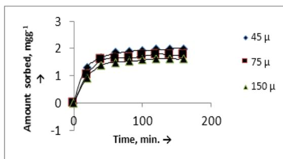
Fig 8: Effect of particle size on adsorption of Cu(II) ion
