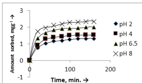
Fig 6: Effect of pH on adsorption of Cu(II) ion
