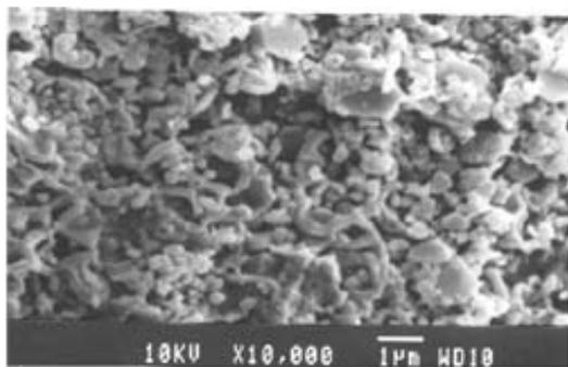
**Fig 2(b):** SEM image of Lead adsorbed CuO sample at high resolution
