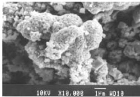
**Fig 3(b):** SEM image of Lead adsorbed NiO sample at high resolution
