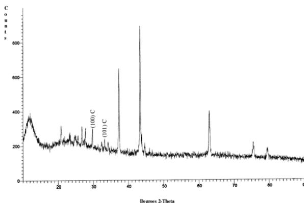
Fig 1(b): XRD Pattern of Lead adsorbed NiO
