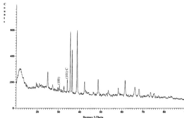
Fig 1(a): XRD Pattern of Lead adsorbed CuO
