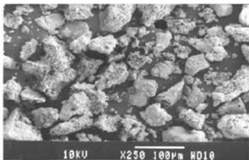
**Fig 2(a):** SEM image of Lead adsorbed CuO sample at low resolution
