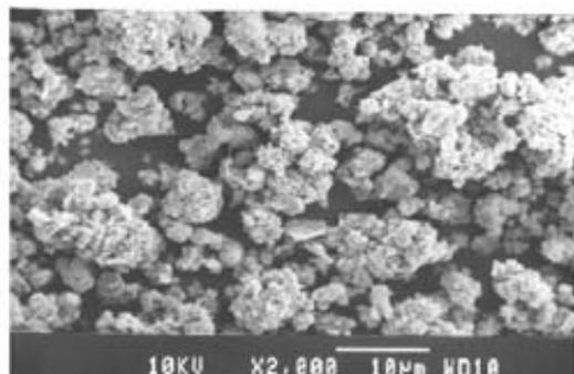
**Fig 3(a):** SEM image of Lead adsorbed NiO sample at low resolution
