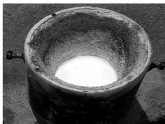
**Fig 2:** Molten charge after aluminothermic reduction process
