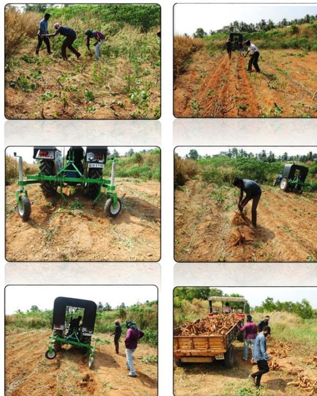
**Fig 3:** Harvesting trials with single row TNAU cassava harvester
