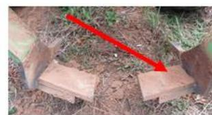
Adjustment of digging blade width
