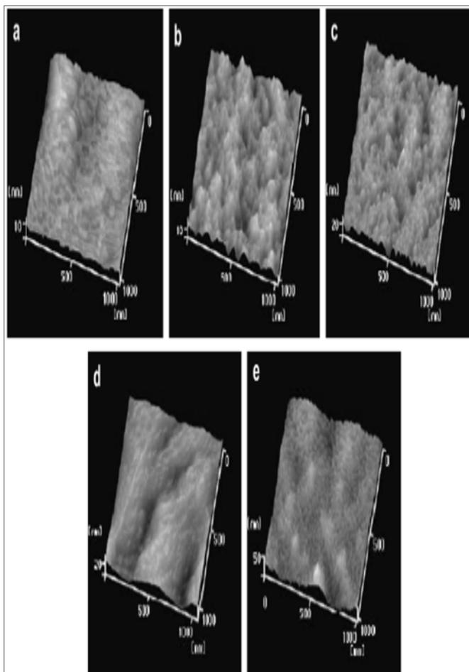
Fig 9: AFM topographic representation of PP film surface for different exposure times: (a) untreated; (b) 5 min; (c) 10 min; (d) 15 min; (e) 20 min (Pandiyaraj *et al.* 2008) [48]
