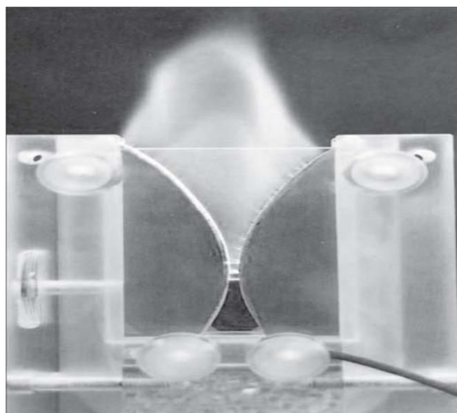
Fig 5: Photo image of the gliding arc in the parallel flow reactor (Fridman et al. 2005) [18]
