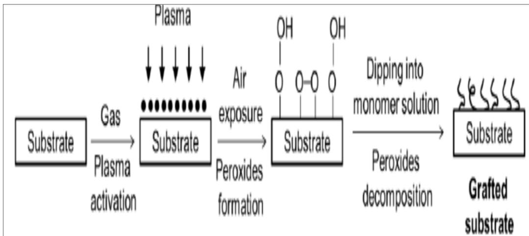
Fig 8: Schematic illustrating the concept of the plasma-induced grafting process (Karam *et al.* 2013) [26]
