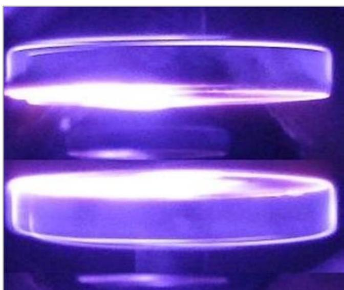
Fig 4: The dielectric barrier plasma discharge (Korachi and aslant, 2013) [30]
