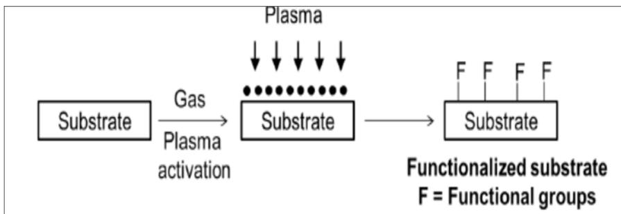
Fig 7: Schematic illustrating the concept of the plasma polymerization process (Karam *et al.* 2)
