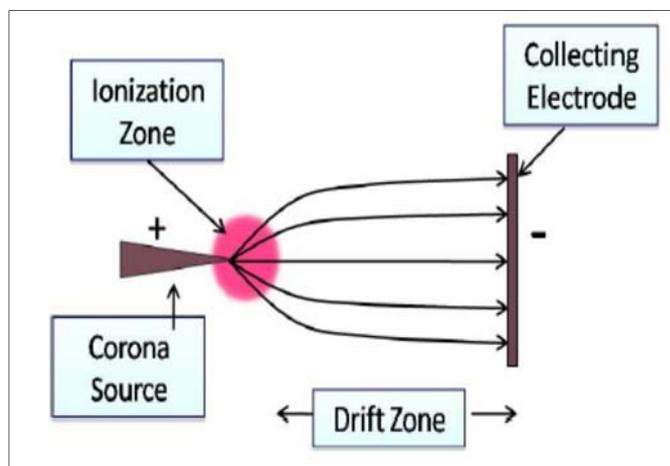
Fig 6: Schematic of a positive corona discharge (Tirumala, 2013) [62]
