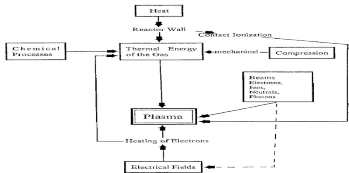
Fig 2: Principles of Plasma generation (Conrads and Schmidt, 2000) [11]
