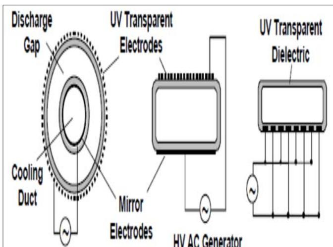
Fig 3: Sealed cylindrical and planar dielectric-barrier discharge excimer lamp configurations (Kogelschatz et al. 1997) [29]
