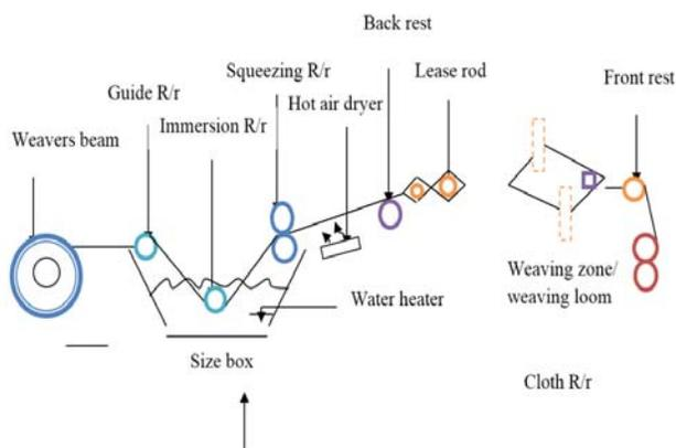
Fig 2.4: Cross sectional view of modified weaving system.
