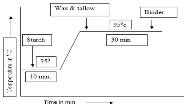
Fig 2.3: Size mixing and cooking procedure
