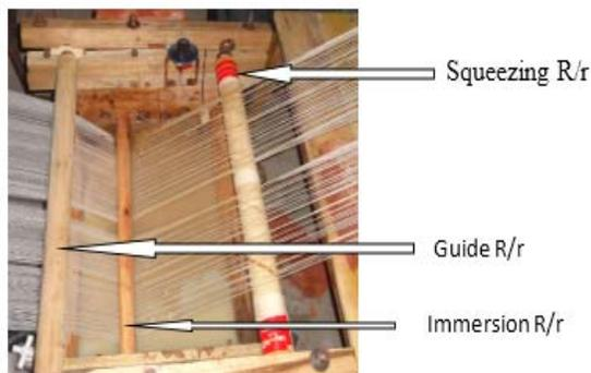
Fig 2.1: New developed wooden size box.
