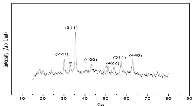
Fig 1: XRD of  $\gamma$ -Fe<sub>2</sub>O<sub>3</sub>
