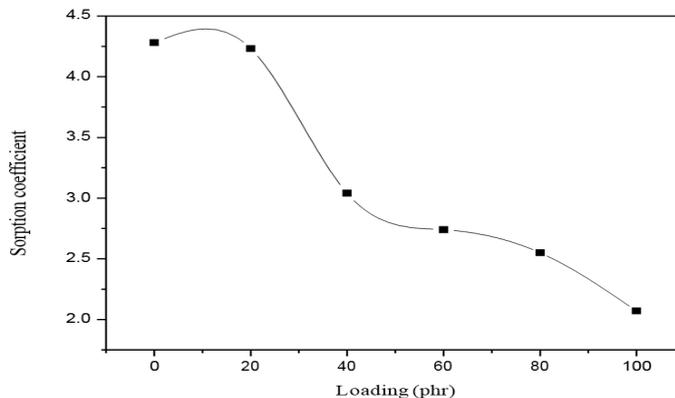
Fig 18: Variation of sorption coefficient with loading
