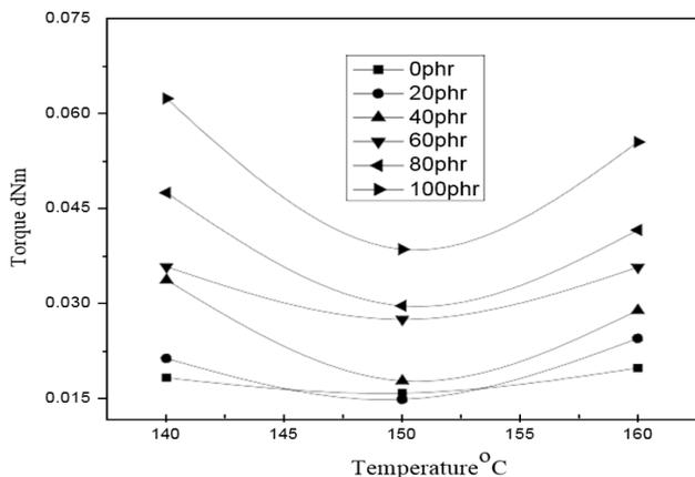
**Fig 8:** Variation in minimum torque with temperature for different loading of the filler
