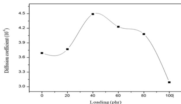
Fig 17: Diffusion coefficients of  $\gamma$ -Fe<sub>2</sub>O<sub>3</sub> filled composites
