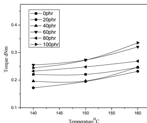
**Fig 7:** Variation in maximum torque with temperature for different loading of the filler
