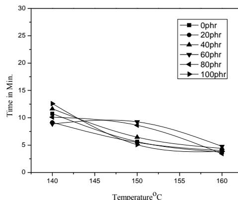
**Fig 5:** Variation of cure time with temperature
