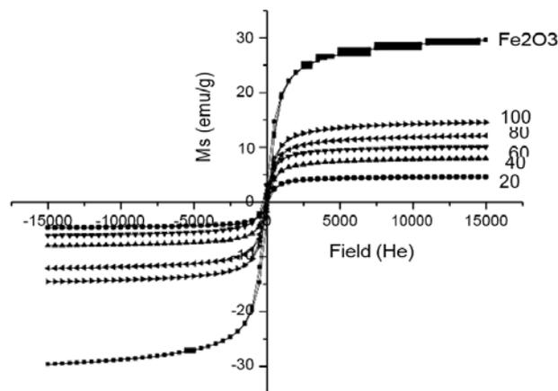
Fig 20: Hysteresis loops of  $\gamma$ -Fe<sub>2</sub>O<sub>3</sub> and composites with different loading of  $\gamma$ -Fe<sub>2</sub>O<sub>3</sub>
