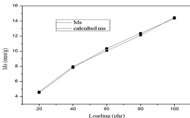
**Fig 21:** Experimental and calculated values of saturation magnetization
