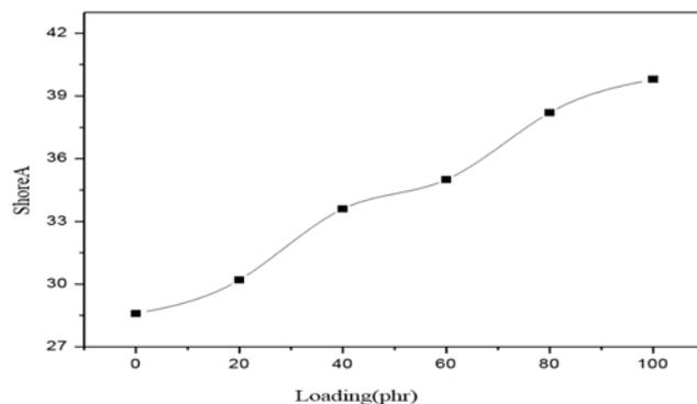
Fig 15: Variation of hardness with filler loading
