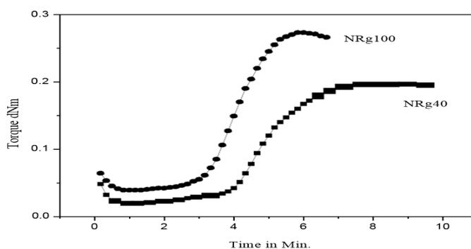
Fig 3: Cure curves for NRg40 and NRg100 at 150 °C
