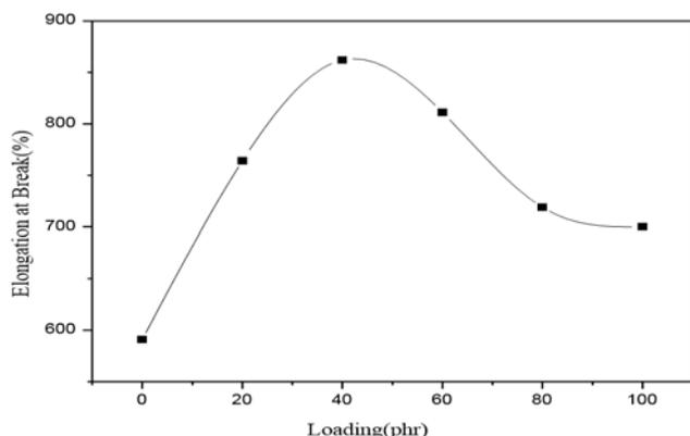
Fig 13: Variation of elongation at break with filler loading
